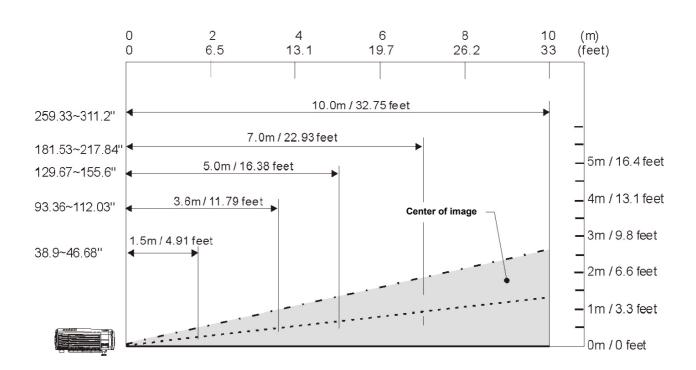
Figure 1: Projection Distance vs. Image Size
